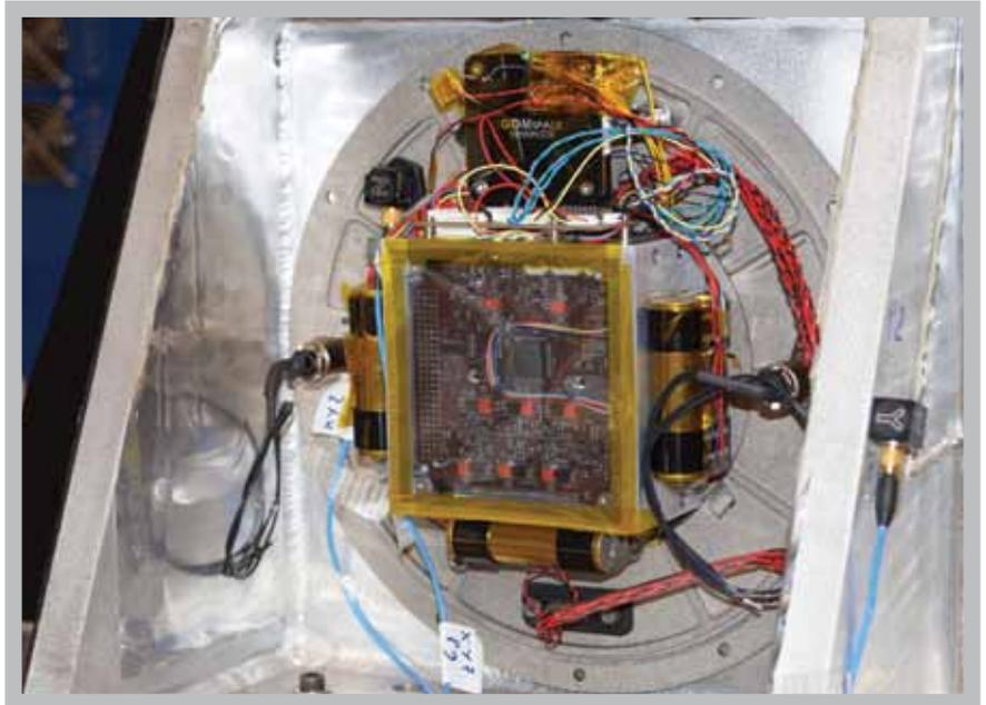
The Engineering and Qualification Model (EQM) of the Demise Observation Capsule on the shaker during testing at CIRA.
